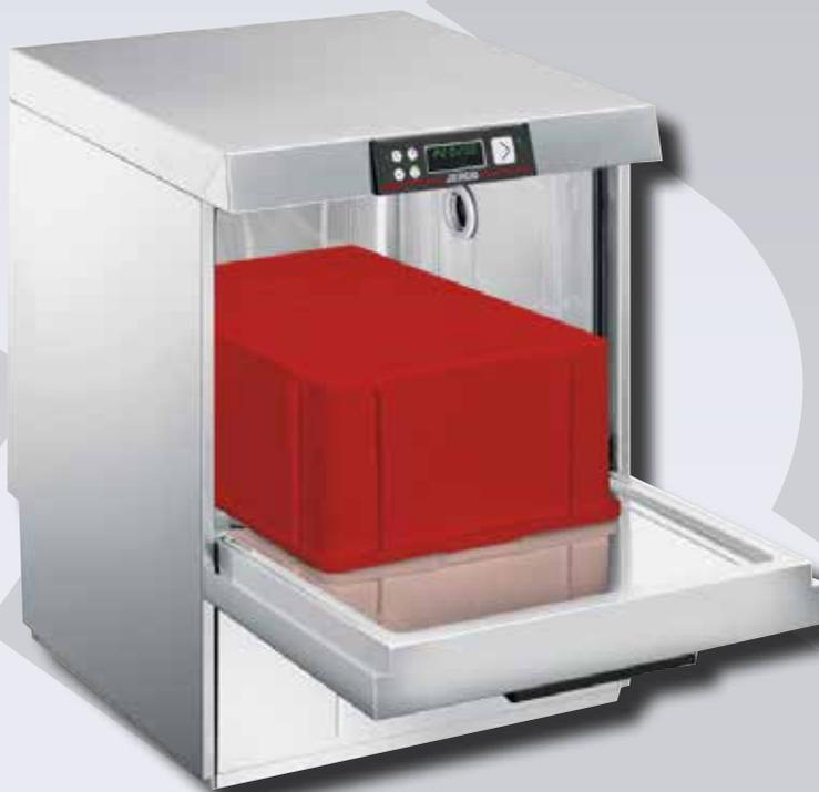
Double skin construction in AISI 304 stainless steel with insulation. Moulded tank with rounded corners. Balanced and insulated door with gasket. 2 rotating wash arms with 8 nozzles each and 2 rinse arms with 7 nozzles each, which is made of stainless steel, ensures optimum washing results.
